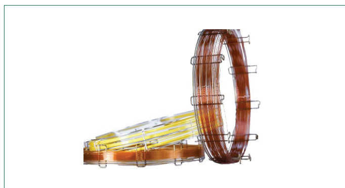
Figure 1: GC Capillary Column.
